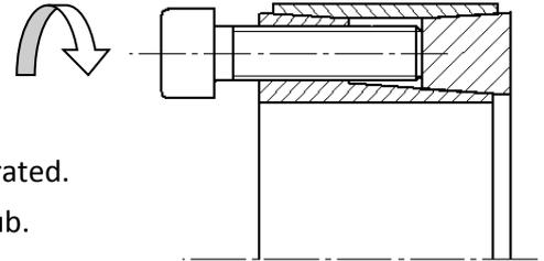
Image 5) Loosening the locking device
