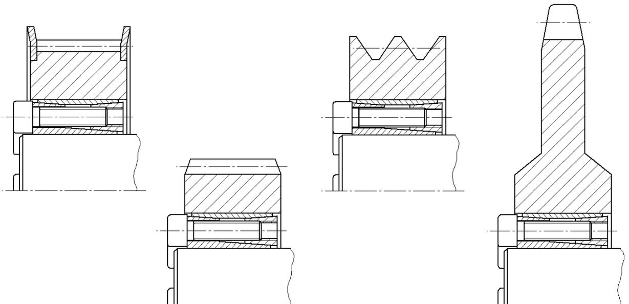
**KBS 52 Locking Device** is a frictionally engaged detachable shaft-hub connection for cylindrical shafts and bores without keyway.
