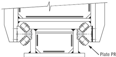
A typical example of Rolbloc system assembly, with opposing parallel guides is shown. For optimal assembly, it is recommended to use adjustment plates PR on one side
