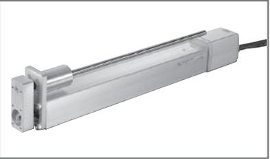
Type Rod (64mm wide) Stroke 50~300mm Load capacity 5kg (horizontal)/24kg (vertical)
