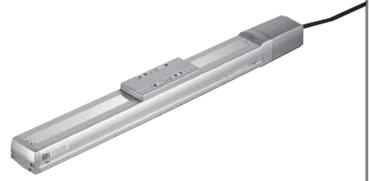
Type Slider (80mm wide) Stroke 100~1000mm Load capacity 55kg (horizontal)/20kg (vertical)
