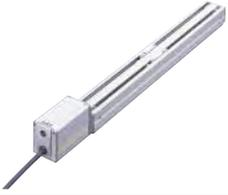
SA6   | A table or other device is installed on the slider to implement movement/positioning in the horizontal or vertical direction. The built-in guides ensure excellent linearity and allow the actuator to accept even an overhung load.                                            | 58                  | 600                 | P15  |
