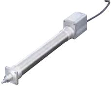
RA54* | A chuck or other device is installed at the tip of the rod that extends/contracts from/into the actuator. Although this type has no built-in guides, external guides can be installed in horizontal applications, or even in vertical applications where linearity is required. | 54                  | 300                 | P17  |
