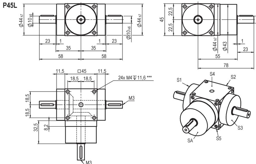
\*) thread starts from 4 mm depth, \*\*) thread starts from 4.5 mm depth, \*\*\*) thread starts from 6 mm depth, feather key to DIN 6885/1
